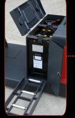
• Optional battery side pull Standard side battery replacement.
