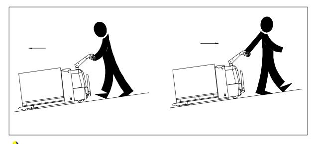
Always keep loads face the downward slope when transport loads on a slope.
