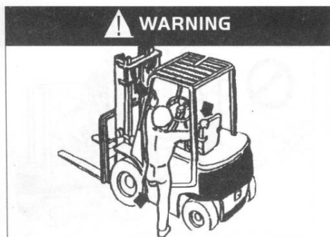
Hold the handrail during on-boarding
