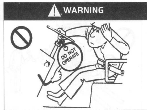
Do not drive an unsafe forklift!
