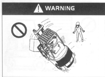
While turning a high speed can cause accident because of unstable center of gravity!
