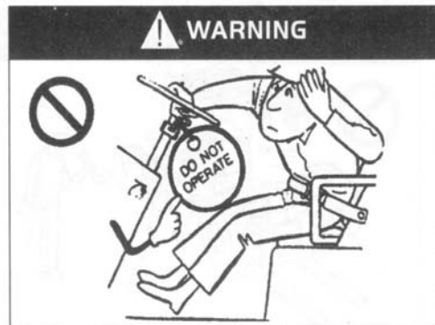
Do not drive an unsafe forklift!
