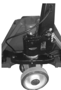
Fig.9: Progressive drive and parking brake
