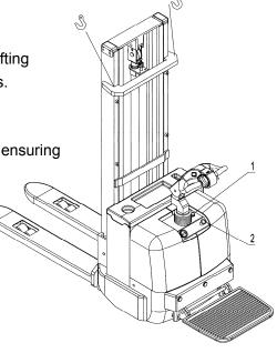
Hooks of the crane must be applied at hook holes, ensuring the stacker will not be slipped down. During operation, make sure the crane, whose hooks must be applied at hook holes of the stacker,
